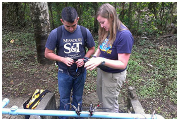
Luis Pereira, left, and Cathryn Pherigo, a senior in chemical engineering, attach a flow meter to a water well in the small village of Santiago, Honduras, during an Engineers Without Borders trip to the Central American country in May.
